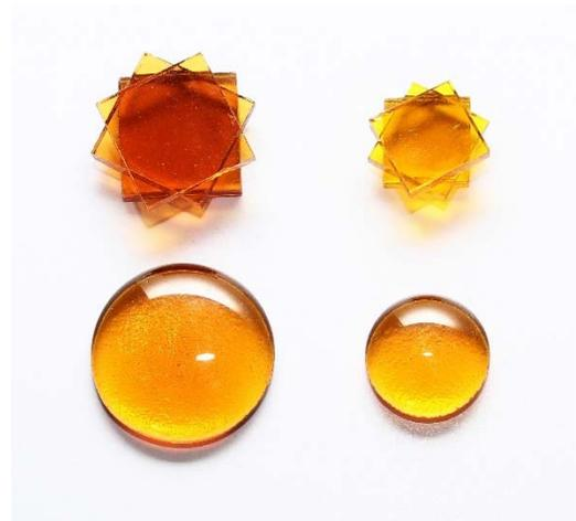
The image on the left is 3 layers of 3/4 inch squares fired to produce a 1 1/8 inch round. The image on the right is 3 layers of 1/2 inch squares fired to produce a 5/8 inch round.
